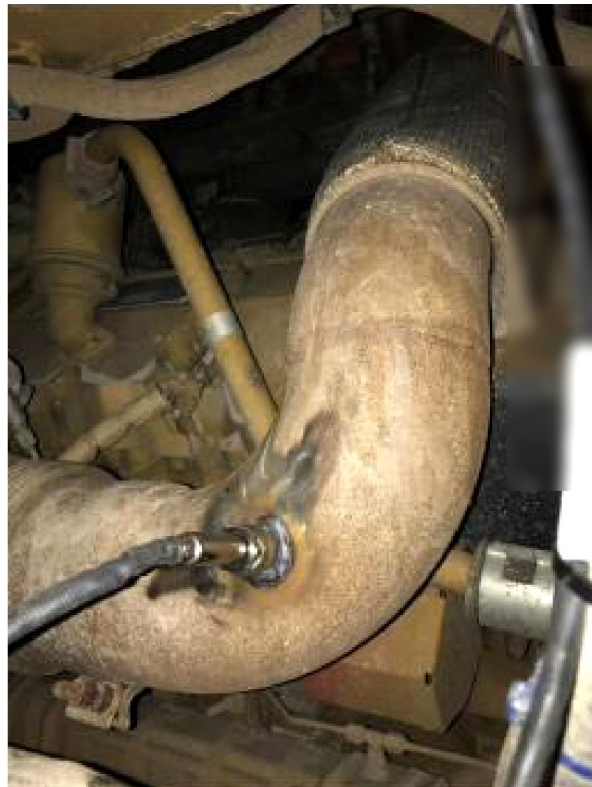
Figure 1: Exhaust gas sampling point at the post-turbocharger location. Field-deployed exhaust sampling at this point captures the direct output of combustion before any aftertreatment chemistry intervenes; on Tier 1 / Tier 2 engines without aftertreatment, it captures unmodified exhaust chemistry. (2018 field deployment context.)
